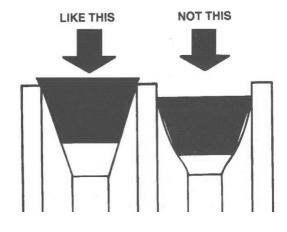
2. Inspect pulleys for wear. Worn pulleys greatly reducbelt life. Extreme wear can lead to belts bottoming in grooves. The result is slippage and excessive heat buildup. Use a pulley groove gauge to check for wear. V-belts should ride at least flush with the top of the pulley and may ride out up to 0.1". Check for burrs, nicks, gouges and severe scratches as these will drastically reduce belt life. Replace if necessary.
