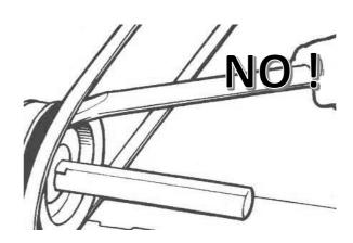
6. Center distance allowances for belt installation and take-up. The center distance should be determined from a standard pitch length and designed so that the centers can be moved closer together and farther apart to allow for installation and tensioning.
