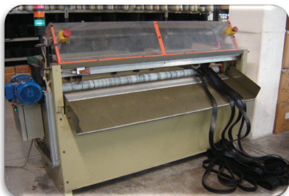
We are equipped to cut rubber sheets into strips and dimension on design.
